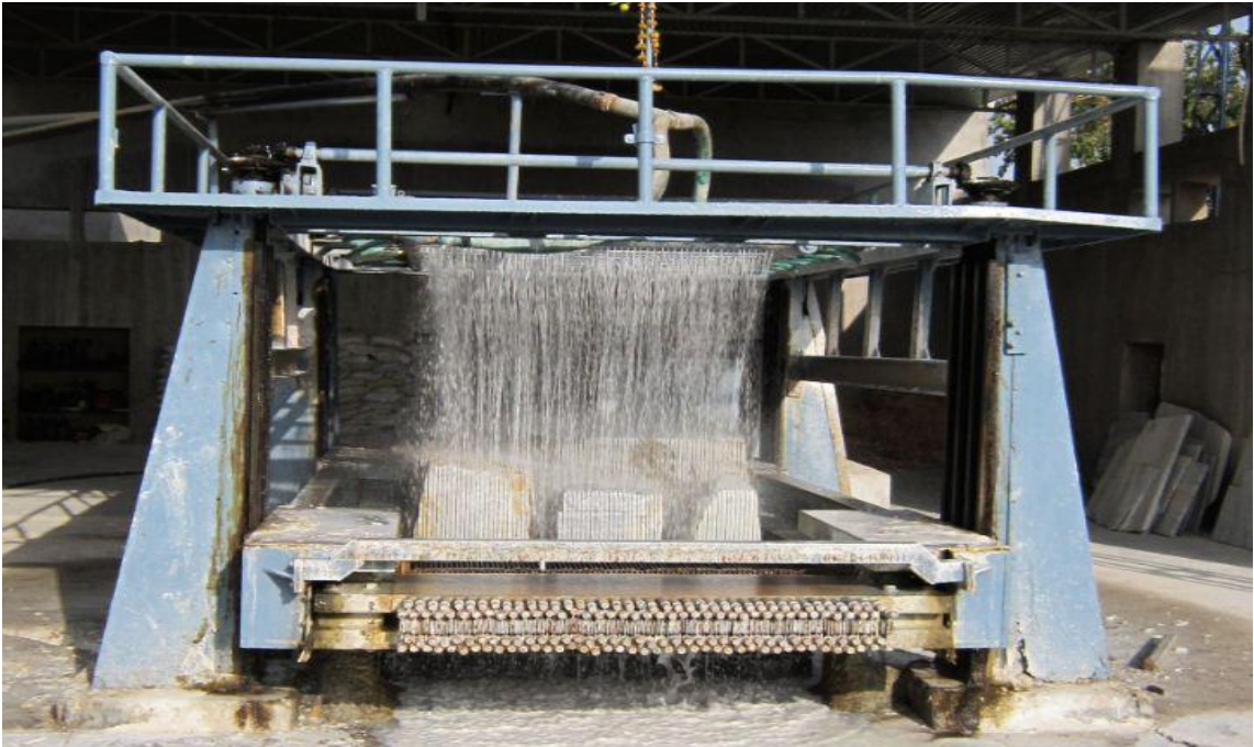
Fig. 4 Processing of Marble Block through Gangsaw machine
