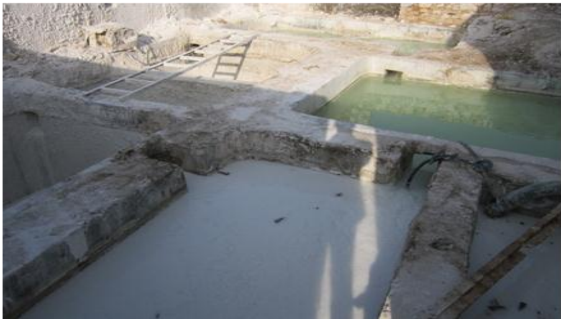
Fig. 5 Sedimentation tanks used for settlement of semi-solid marble slurry
